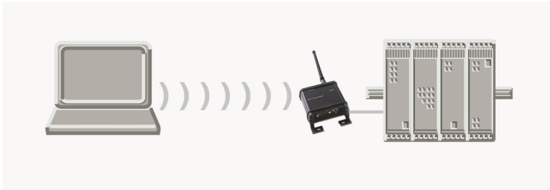
Caption: PC-based programming tool connected to a Programmable Logic Controller (PLC) with a serial cable replacement
