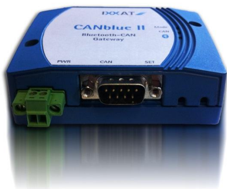
Caption: There is a large variety of fieldbuses in the industry that are either standard or vendor specific fieldbuses. An example of such a device is a CAN / Bluetooth Adapter.
