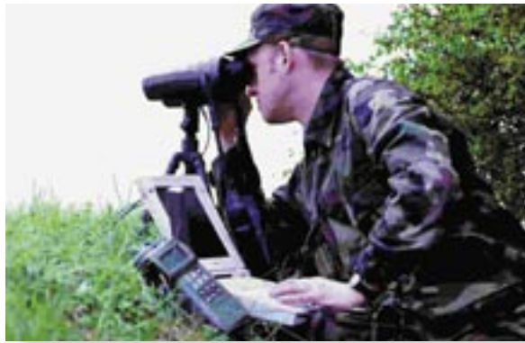
The Serial Port Adapter provides reliable system transfer measuring data from the VECTOR binocular to the PDA.
