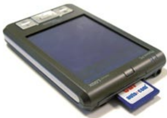
CDP, Compact Diagnostic Partner, is a userfriendly Bluetooth based tool for car-specific diagnostics.
